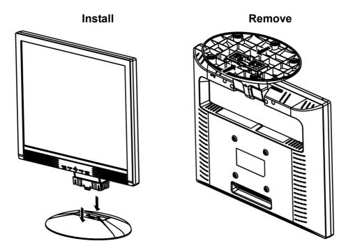
Figure.1. Installing and Removing the Base
